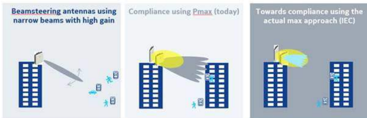
Picture: Difference in safety distance assessment using Pmax and actual max approach
